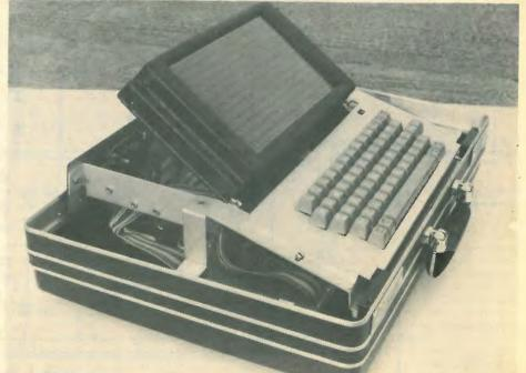
selected because its bipolar technology renders An early prototype of the Microdata model 8400 briefcase computer, now going into production.
