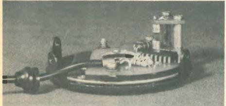
Fig. 4. Phototransistor and I.e.d. mounting. The two pillars must be metal types to carry the I.e.d. current.
